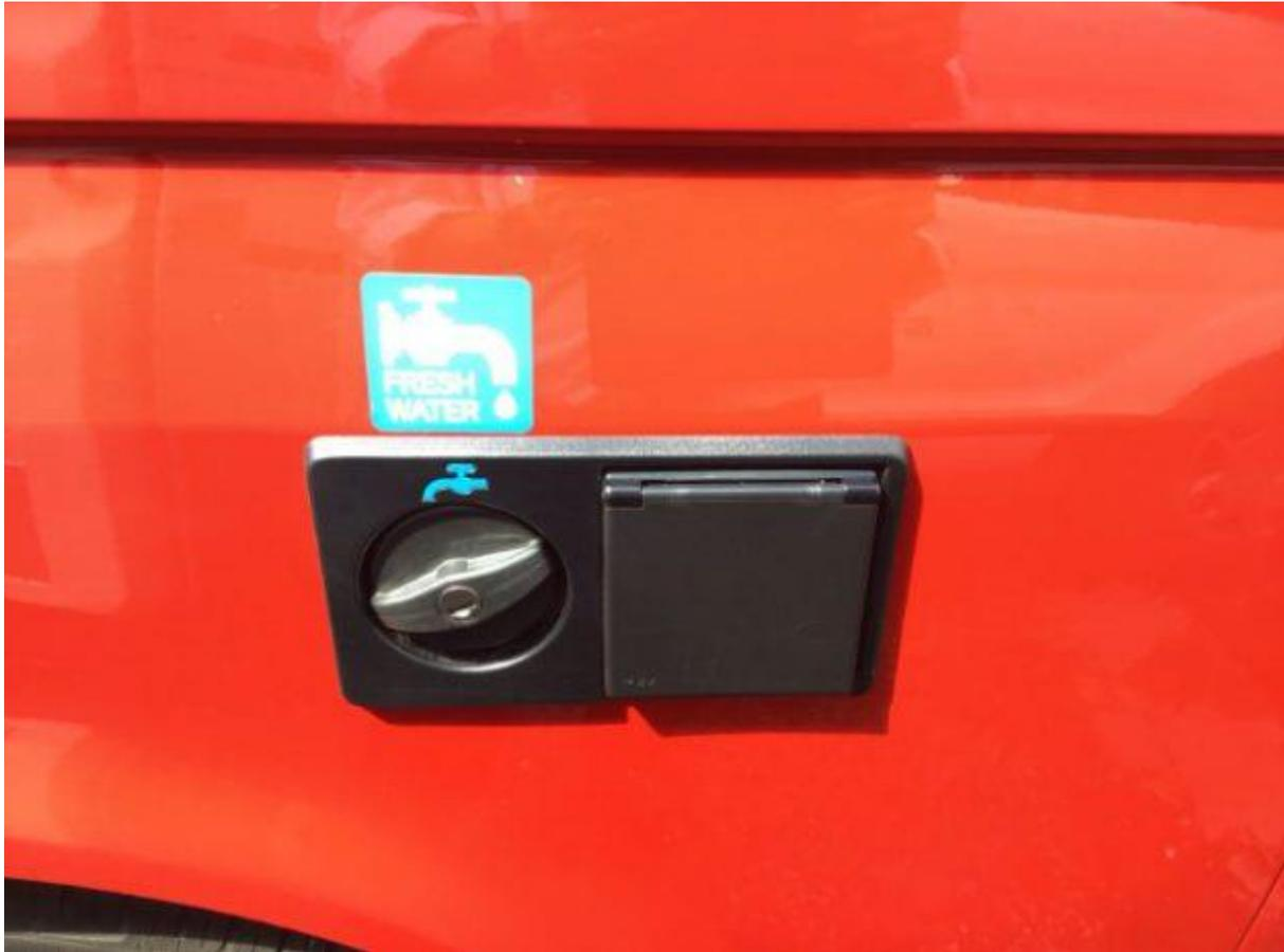
The flap for the electric hook up is on the left next to water point.
