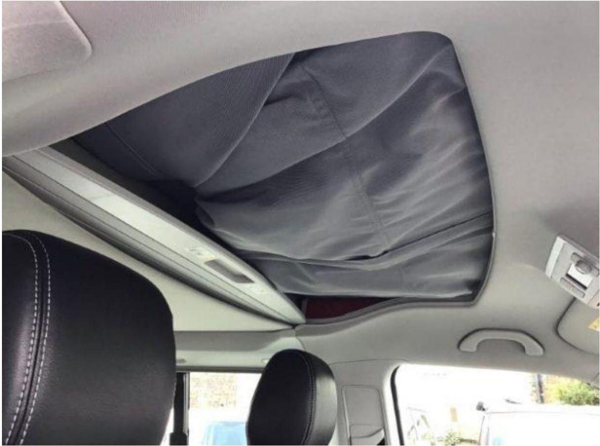
1. Check that the upstairs area is clear of bedding, pillows, everything except the mattress that belongs up there. If articles are left in this area then the roof will not close properly and it will damage and twist the roof.
