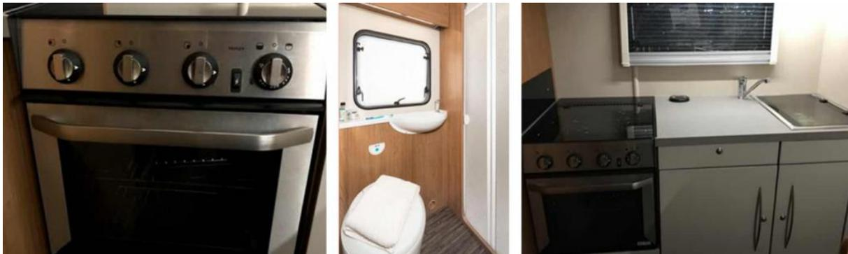
The vehicle also has a shower and toilet, also there is a 135 litre fresh water tank providing cold running water in the kitchen and bathroom. Hot water and central heating for the vehicle is powered by LPG (Liquid Petroleum Gas). LPG can only be used when the vehicle is static.
