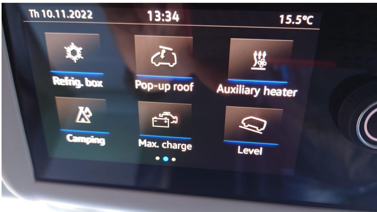
Switch on pressing the box next to switch on Refrig box you will see the ice symbol appear
